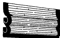
Notes: The Edge Banding will show on the bottom hem even when the shade is in the raised position.
