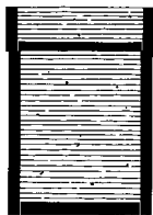
Both Sides and Hems - BSH4 (Bottom hem has 3" banding to cover weight bar inserted in hem)
